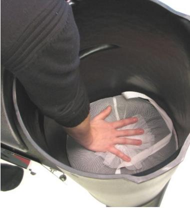
*Push the element down until all the trapped air has escaped out of the carbon element.*
