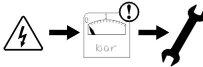
2. Depressurise the system before installation or maintenance is carried out!
