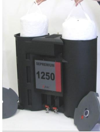
13. Replace both lids. (Lid 1 on tower 1 and lid 2 on tower 2). The static white element will be pushed in place by lid 2.
